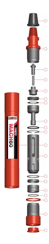
G. Grease threads and screw Drill Bit (19), Chuck (18), Chuck Spacer (17) and Bit Retaining Ring (15) into bottom of Cylinder (11).
