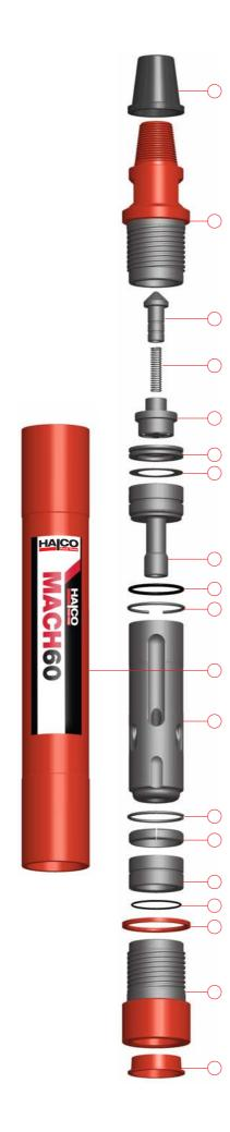
D. Remove Chuck Spacer (17) from Chuck (18). Remove Bit Retaining Rings (15) from Drill Bit (19) and remove 'O' Ring (16) from Bit Retaining Rings (15).
