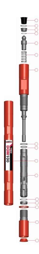
**D.** Grease splines and fit Chuck (15) over Drill Bit (16).
