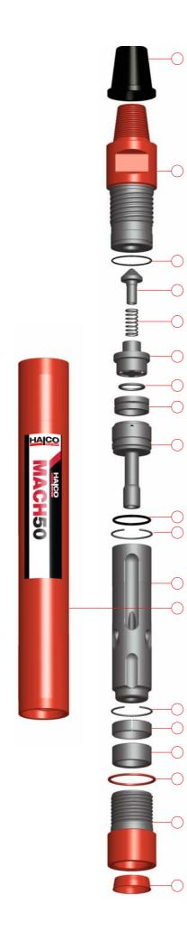
**E.** Grease splines and fit Chuck (18) onto Drill Bit (19).
