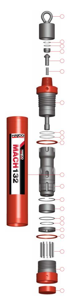
**D.** Remove Chuck Spacer (18) from Chuck (20). Remove Bit Retaining Rings (17) from Drill Bit (21) and remove Containment Band (16) from Bit Retaining Rings (17).
