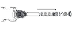
L. Unscrew and remove Top Adaptor (8) from Cylinder (11).
