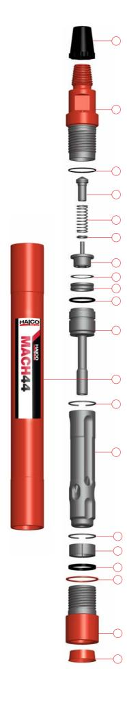
G. Coat Piston (14) liberally with rock oil minimum 200 centistroke and insert into top of Cylinder (13) ensure it is inserted the right way round as illustrated.
