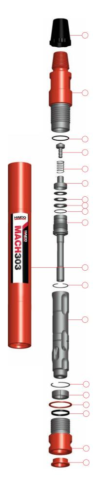
**E.** Place Chuck Spacer (18) over Chuck (19) and place Bit Retaining Rings (16) over Drill Bit (20).
