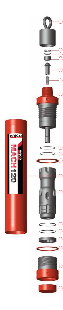
**E.** Fit Chuck Spacer (16) onto Chuck (17). Fit Containment Band (14) onto Bit Retaining Rings (15) and fit Bit Retaining Rings (15) onto Drill Bit (18).
