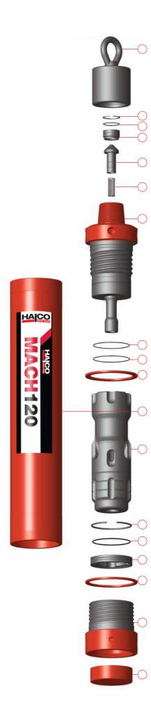
**D.** Remove Chuck Spacer (16) from Chuck (17). Remove Bit Retaining Rings (15) from Drill Bit (18) and remove Containment Band (14) from Bit Retaining Rings (15).
