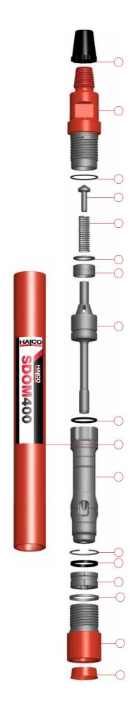
**F.** If required fit Containment Band (13) onto Bit Retaining Rings (14). Fit Bit Retaining Rings (14) onto Drill Bit (17).
