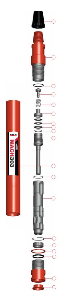
**D.** Remove Bit Retaining Rings (16) from Drill Bit (20) and Chuck Spacer (18) from Chuck (19).
