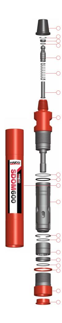
**D.** Remove Chuck Spacer (19) from Chuck (20). Remove Bit Retaining Rings (17) from Drill Bit (21) and remove 'O' Ring (18) from Bit Retaining Rings (17).
