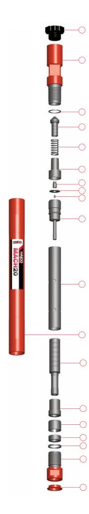
**D.** Oil Piston (13) and insert piston shank into Piston Guide Bush (14). Then slide Liner (11) with air holes nearest the end first over Piston (13) and up against the shoulder of Piston Guide Bush (14).
