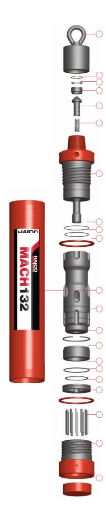
E. Insert 'O' Ring (15) into bottom of Cylinder (11) ensure it seats in the internal 'O' ring groove.
