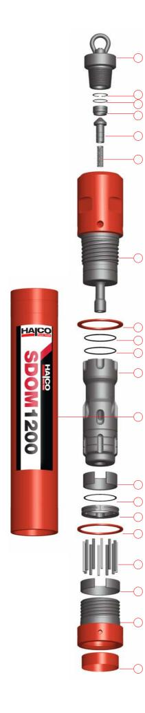
E. Grease spline and fit Chuck (19) onto Drill Bit (20). Insert Drive Pins (17) between Drill Bit (20) and Chuck (19) splines.
