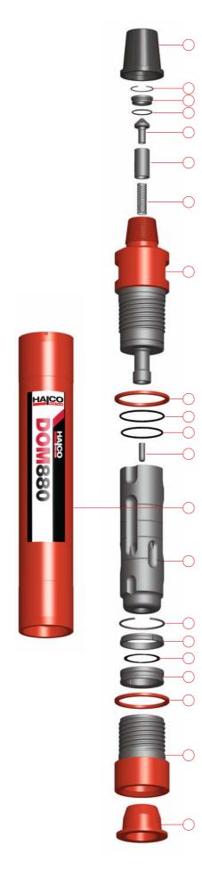
**D.** Remove Chuck Spacer (19) from Chuck (20). Remove Bit Retaining Rings (18) from Drill Bit (21) and remove Containment Band (17) from Bit Retaining Rings (18).
