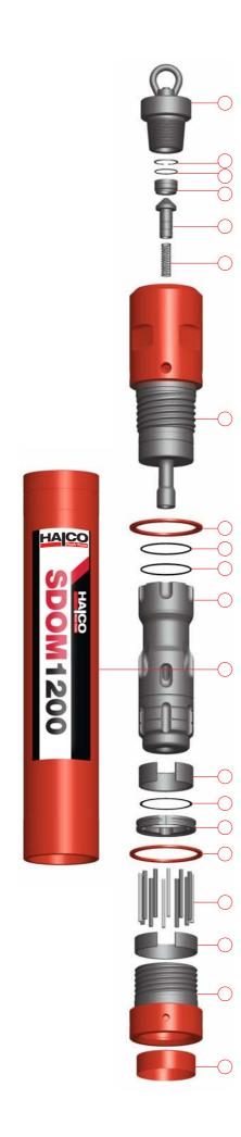
D. Remove Chuck Spacer (16) from Chuck (19). Remove Bit Retaining Rings (15) from Drill Bit (20) and remove Containment Band (14) from Bit Retaining Rings (15).
