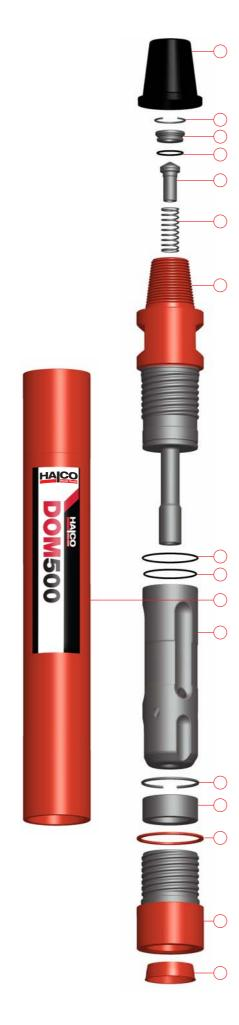
**E.** Fit Chuck Spacer (16) over Chuck (17) and fit Bit Retaining Rings (14) over Drill Bit (18).
