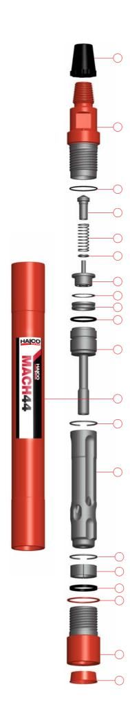
D. Remove Chuck Spacer (18) from Chuck (19) and remove Bit Retaining Rings (17) from Drill Bit (20).
