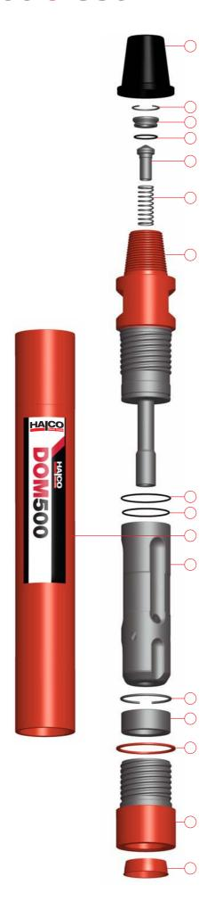
**D.** Remove Chuck Spacer (16) from Chuck (17) and remove Bit Retaining Rings (14) from Drill Bit (18).
