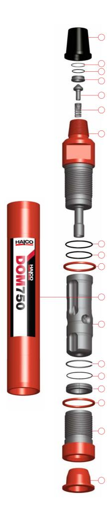
**E.** Fit Chuck Spacer (16) onto Chuck (17), Fit 'O' Ring (14) onto Bit Retaining Rings (15) ensure it seats in the 'O' Ring groove. Fit Bit Retaining Rings (15) onto Drill Bit (18).
