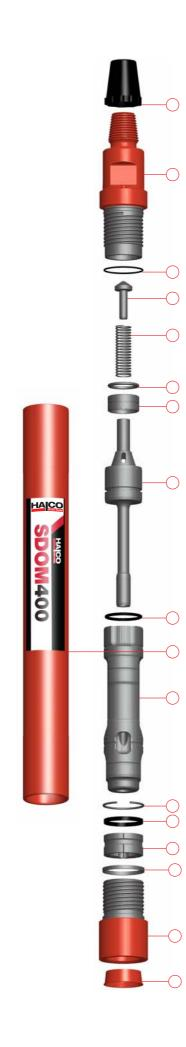
**D.** Remove Bit Retaining Rings (14) from Drill Bit (17). Remove Containment Band (13) if fitted from Bit Retaining Rings (14).
