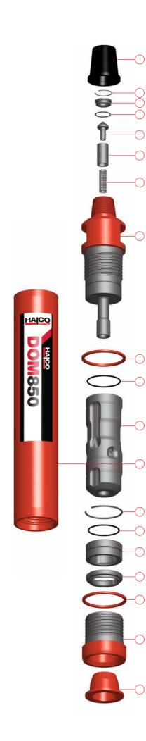
D. Remove Chuck Spacer (17) from Chuck (28). Remove Bit Retaining Ring (16) from Drill Bit
