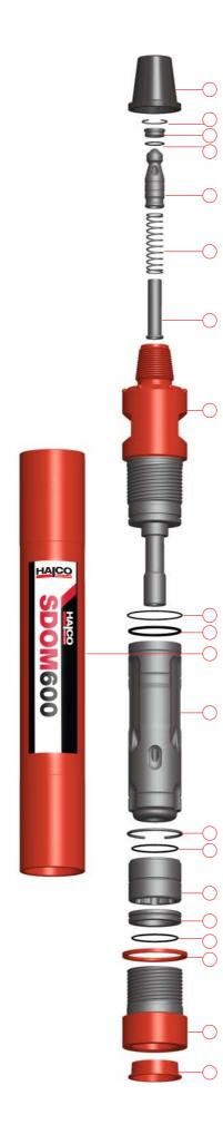
**E.** Fit 'O' Ring (15) onto Bit Guide Bush (16) ensure it seats in the 'O' Ring groove. Insert Bit Guide Bush (16) into bottom of Cylinder (11).
