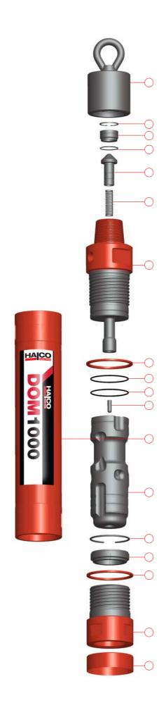
**D.** Remove Chuck Spacer (16) from Chuck (17). Remove Bit Retaining Rings (15) from Drill Bit (18).
