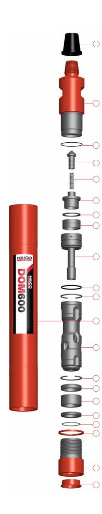
E. Remove Chuck (20) from Drill Bit (21).
