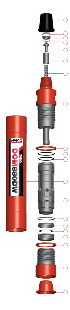
E. Grease splines and fit Chuck (20) onto Drill Bit (21).
